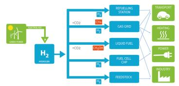
hydrogen can be used for transportation, power generation, heating, and industry. This is referred to as Power-to-X (P2X).<sup>5</sup> When the electrolytic hydrogen is used for power generation, the function is identical to a battery but with the potential for storage of massive amounts of energy for any duration of time from hours to seasons. In non-power applications, electrolyzers can serve as a flexible load having similar benefits to traditional storage resources.
