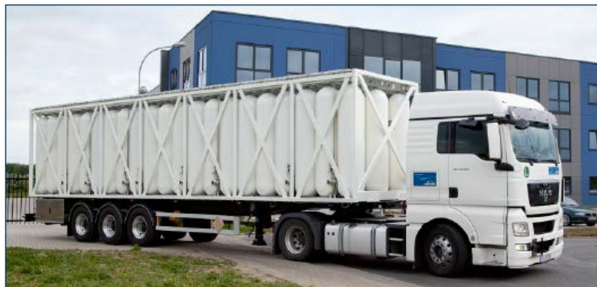
Figure 8: Linde 500 bar trailer with 1,100 kg of hydrogen capacity
