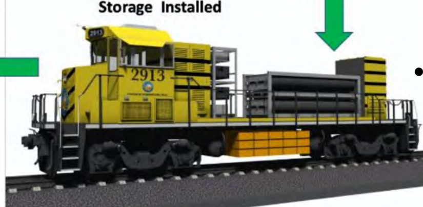
Repowered with 200 kW Fuels Cells, 222 kg Hydrogen Storage, and 500 kW-hr Battery Storage Installed
