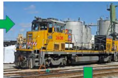
RP20BD With Diesel Engine Pods Removed
