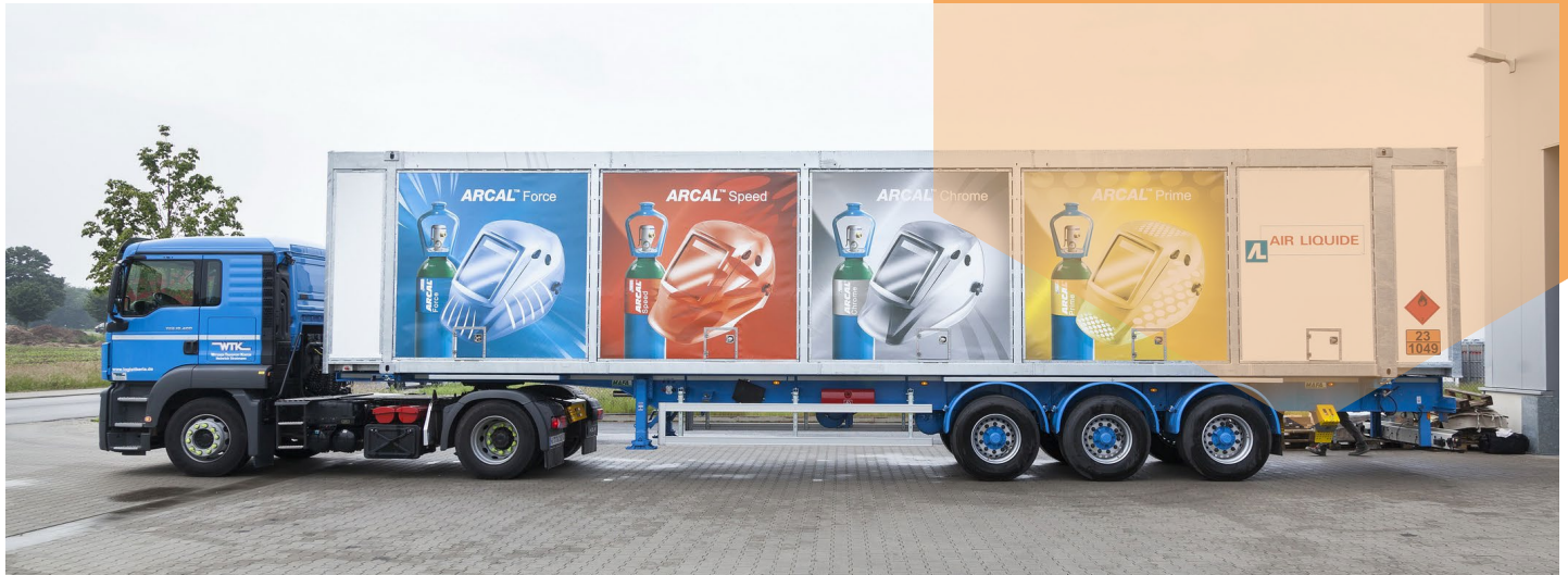
Our X-STORE® modules are available as containerized or trailer solutions. (photo: 45 ft ISO container for hydrogen from Air Liquide)
