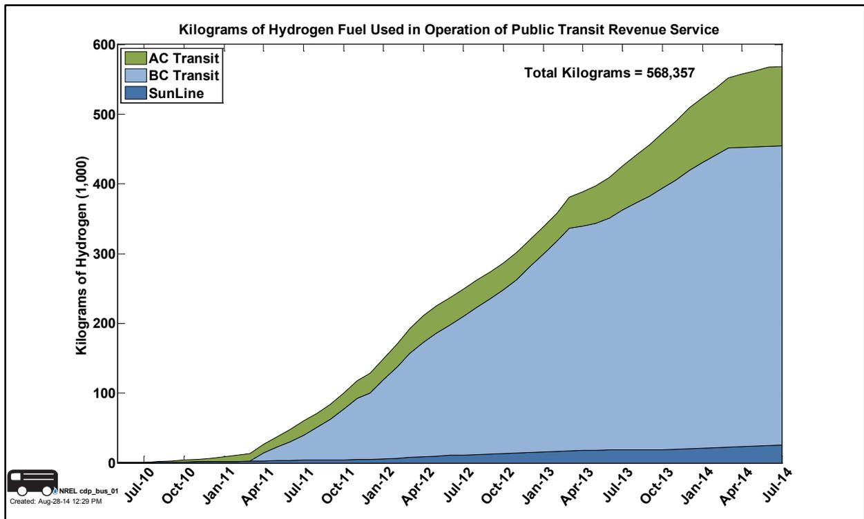
Figure 9. Hydrogen dispensed for the FCEBs through July 2014
