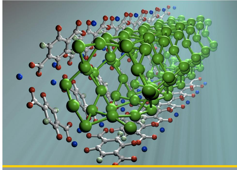
Hydrogen can be stored on the surfaces of solids by adsorption. In adsorption, hydrogen associates with the surface of a material either as hydrogen molecules ( $H_2$ ) or hydrogen atoms (H). This figure depicts hydrogen adsorption within MOF-74.
